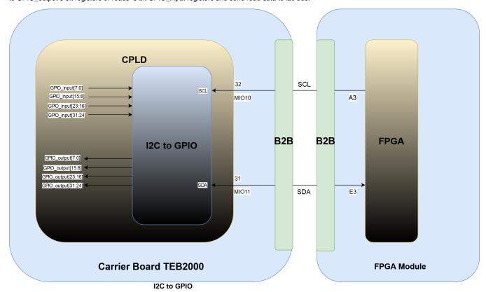
I2C bus is connected to MIO10 ( SCL signal) and MIO11 (SDA signal). MIO10 to MIO15 are direct connection between CPLD of TEB2000 and FPGA on the module (for example TEM0007) through B2B connector. If in FPGA design exists no i2c interface for MIO10 and MIO11, this block will be unused. More information about MIO10 to MIO15 are shown in the following table for TEM0007 modules and TEB2000 carrier board:
