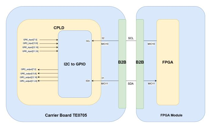
I2C bus is connected to MIO10 (SCL signal) and MIO11 (SDA signal). MIO10 to MIO15 are direct connection between CPLD of TE0705 and FPGA on the module through B2B connector. If in FPGA design exists no i2c interface for MIO10 and MIO11, this block will be unused. More information about MIO10 to MIO15 are shown in the following table for whole Trenz Electronic 4x5 modules and TE0705 carrier board:
