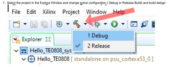
2. To build selected configuration again, use build symbol or right click on the application project in the Explore Window and press "Build Project" or "Clean Project" to generate/regenerate the application project elf files
