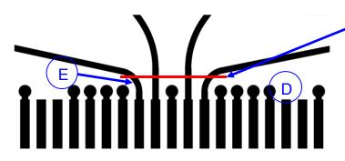
Measurement reference plane for the ST5 connector side
