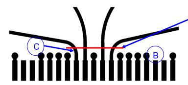
Measurement reference plane for the SS5 connector side
