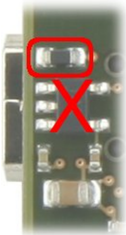
Assembly option for VCCAUX = 3.3 V (bottom view).
