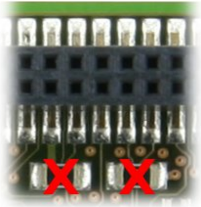
Assembly option for VCCAUX = off (bottom view)
