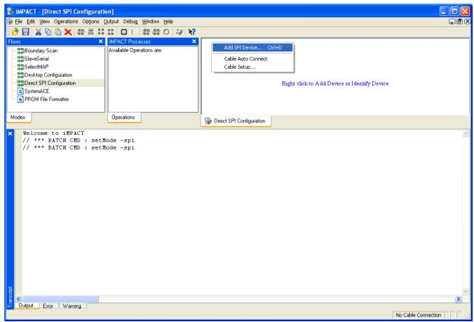
Right click the "Direct SPI Configuration" panel to add a device and select "Add SPI Device"
