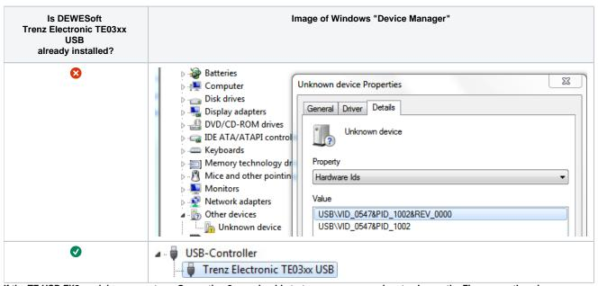
If the TE USB FX2 module enumerate as Generation 2 you should start a recovery procedure to change the Firmware, otherwise you may need to install the Generation 2 driver.
