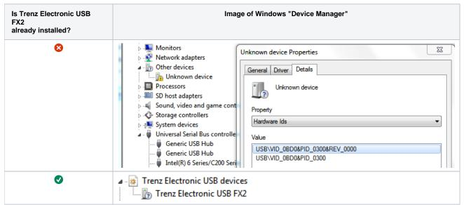
If the TE USB FX2 module enumerate as Generation 3 you should check if the Trenz Electronic USB FX2 device driver is already installed; if it is already installed the procedure ends here.
