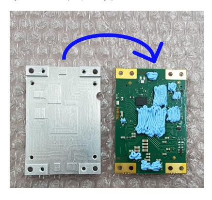
Set the torque screwdriver to 0.5Nm.Insert the PH1 Philips crosshead bit and fix it crosswise from below with the four M3x6mm pan-head screws.
