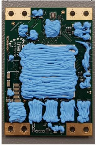
2. Align KK0808-03 carefully and press on lightly:
