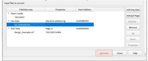
You can use the Quartus Programmer to program the flash configuration device with the .jic file.
