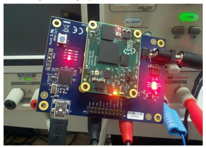
LED blink with TCL magic. There are actually 3 LED's blinking, the "Vivado TCL" LED is the red LED at the far top of TE0710.
