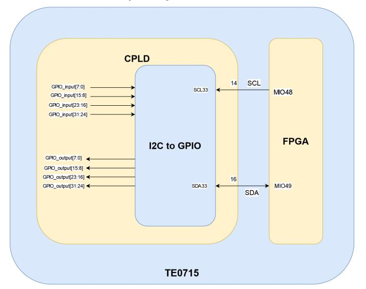
I2C to GPIO is used to set boot mode in linux console or in FSBL code. It is used to activate boundary scan mode too.
