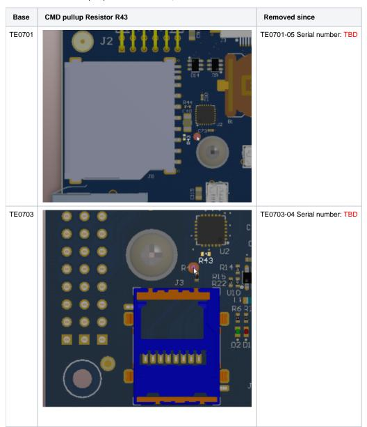
This extra pullup may cause problems in some special cases with some SD Cards. As example hama micro-SD Card when used with PS7 SDIO MIO pullups enabled and R43 loaded had sporadic initialization problems on TE0703, removing R43 solved the issue.
