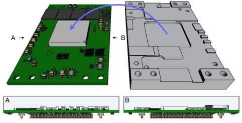
Set the torque screwdriver to 0.5Nm / 4.5 inlb.
