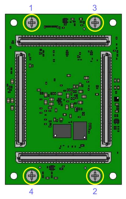
5. Fasten the heatspreader crosswise from below with the four M3  $\times$  6 mm pan-head screws.
