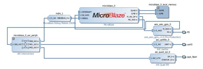
Example ASIO Demo for TE0711 SoM: a total of 196 I/O pins are connected to single ASIO GPIO IP Core. All ports are mapped to FPGA pins using Vivado board part flow, no manual constraints entered.
