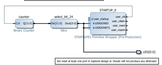
$Blink\ a\ LED,\ this\ design\ will\ work\ on\ ANY\ Artix,\ Kintex,\ Virtex\ or\ Zynq\ Board\ and\ Blink\ DONE\ pin\ and\ one\ I/O\ pin.$
