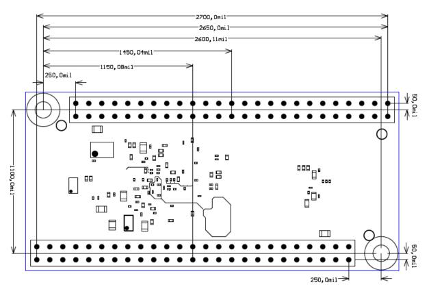
All 100 mil pin headers are in 100 mil grid, the M3 mounting holes are in 50 mil grid aligned to the centers of the 100mil headers. The module is symmetrical, turning it 180 degrees will keep all I/O and Power pins in both 50 pin headers in compatible places.
