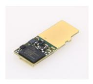
TE0747 is a MicroSD Card sized (over-sized in length) Programmable Platform capable to be used as Google Project Vault device or as generic SD Card Emulation Device. TE0747 can also be used with custom Protocols or switched device that can be accessed as SD Card first to transfer files to on-board NAND, then later the microSD card edge terminals can be used as user I/O for other purposes.
