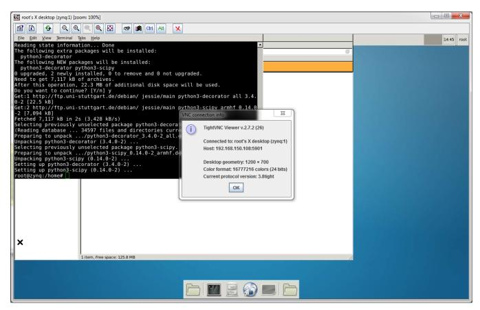
VNC session to Remote desktop on TE0720 (without any actual display device). Similarly remote desktop access is possible to any other Zynq based system or SoM with Ethernet connection and external RAM.
