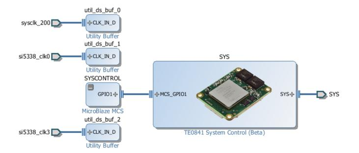
All Interfaces visible are connected by Vivadi Board automation, the SYS interface includes all TE0841 fixed on-board connections that the System Controller manages. SYSCONTROL is a small MicroBlaze MCS based controller that does initialize the Si5338 PLL Multisynth and can perform other functions as well.
