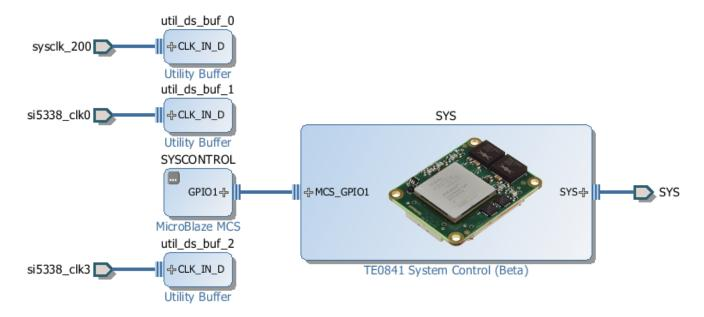
All Interfaces visible are connected by Vivadi Board automation, the SYS interface includes all TE0841 fixed on-board connections that the System Controller manages. SYSCONTROL is a small MicroBlaze MCS based controller that does initialize the Si5338 PLL Multisynth and can perform other functions as well.
