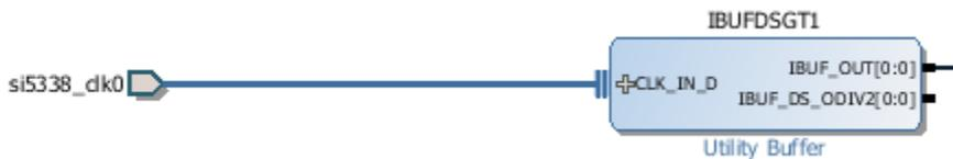
Clock buffers for GT Clock in Xilinx 7 Series Devices (example from TE0745 design)
