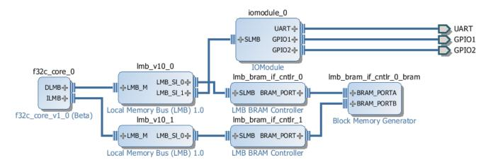
Example F32C SoC using IOModule from Vivado IP Catalog, again the addresses for BRAM and the IOModule are assigned automatically and can be changed as needed in Address Editor.
