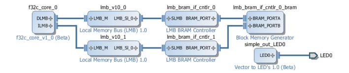
Data and Instruction buses are exported as LMB Bus, then IPI Standard IP cores are used to add BRAM. The size of the BRAM can be selected in the Address Editor:
