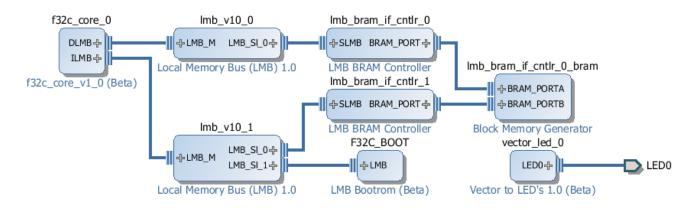
LMB Bootrom IP Core added with fixed code for the bootstrap.
