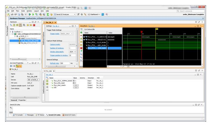
Debug session in Vivado Labtools, when CPU Reset is asserted Instruction address bus freezes, but after release there seems to be no reset, F32C Core tries to continue from last PC Address.
