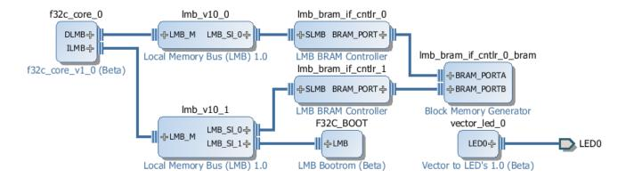
LMB Bootrom IP Core added with fixed code for the bootstrap.
