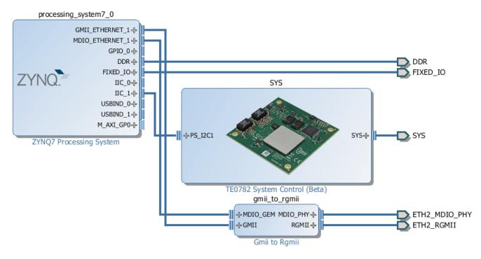
Example use of the SC0782 IP Core, this IP Core pulls its I/O connection from Board Part files automatically without any need to add XDC constraints manually. This IP Core can control and/or forward fixed I/O connections on the TE0782, those fixed connections are encapsulated in one single SYS interface to make the Block Diagram more readable.
