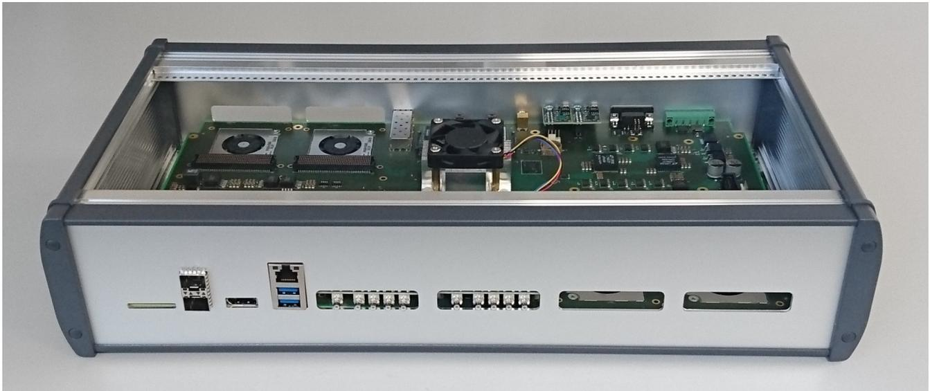
UltraRack+ with 2 L-BAND SDR FMC Cards, still 4 FMC free, 2 front, 2 back of the rack.
