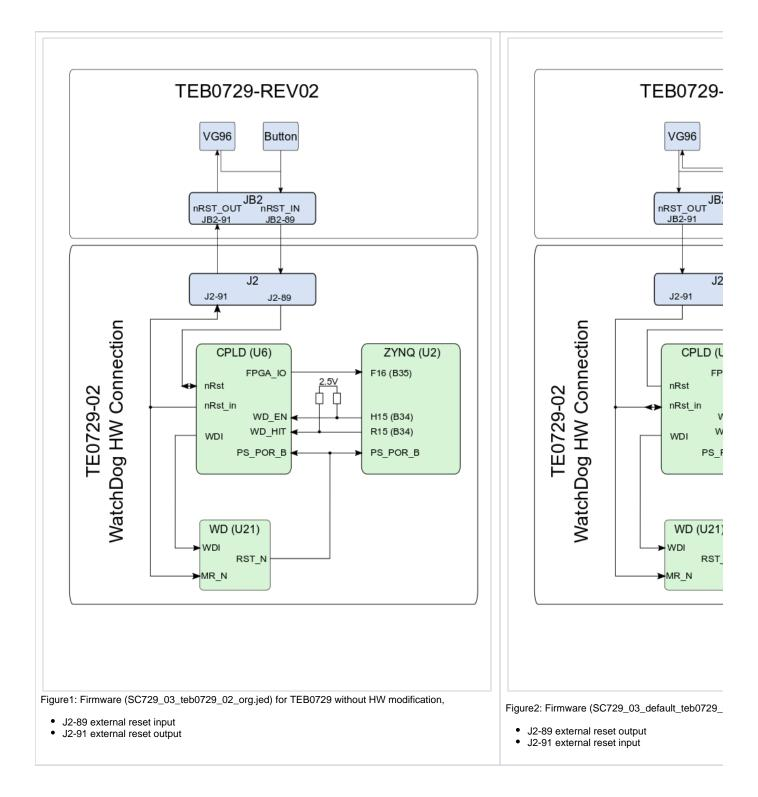
2 Variant available, depends on carrier board connection, see Figure 1 and 2. The swapped signals and nRST\_IN pulse limitation on variant 1 are the only difference between this two variants.
