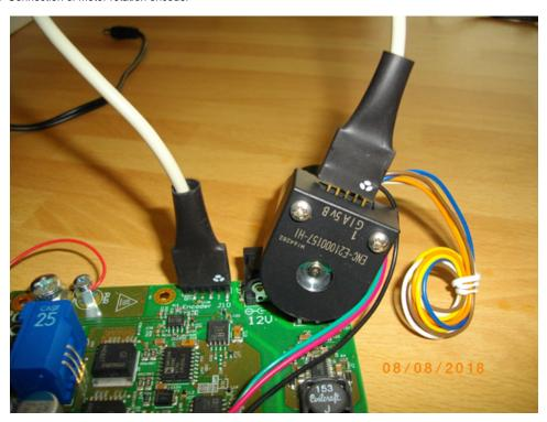
Motor rotation encoder is connected to the TEC0053-04 - EDPS Power Stage Pmod 6 pin cable connector kit. See the orientation and position of the 5 wire connection. There are 6 pins on the TEC0053-04 board. There are only 5 pins on the motor encoder. Pin 1 connects to pin 1. 6-th wire is unconnected on the motor encoder side.
