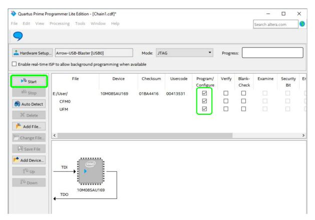
Mark the "Program/Configure" box for the selected file. The programming of the FPGA is executed, when you press the button "Start". When the programming finishes, the Quartus Prime Programmer can be closed.
