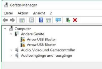
Through a right mouse click on each device, a context menu opens. Chose "**Update driver**" afterwords chose "**Search automatically for updated driver software**", this proper driver installation changes the devices names into USB Serial Converter A & B, in addition, also the comport is installed.
