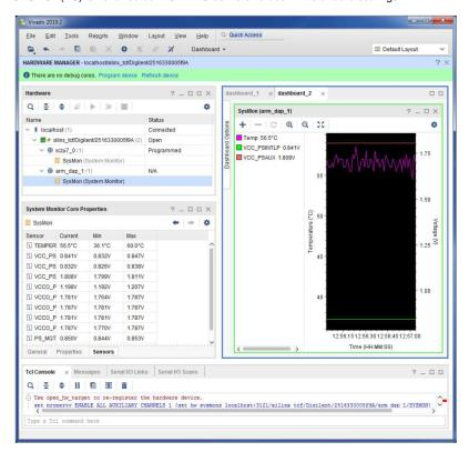
Workaround: Either use scale factor 1.5 when using PL XADC or simple only use readings from PS XADC.
